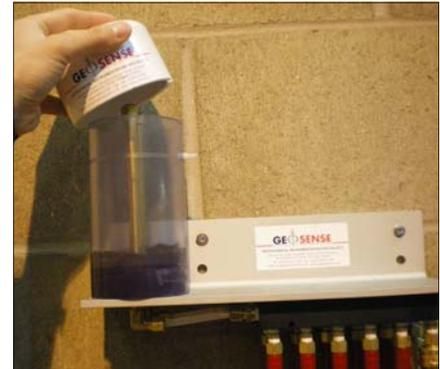
13. Remove the nuts to release liquid and add more liquid to make up to the overflow level again.
