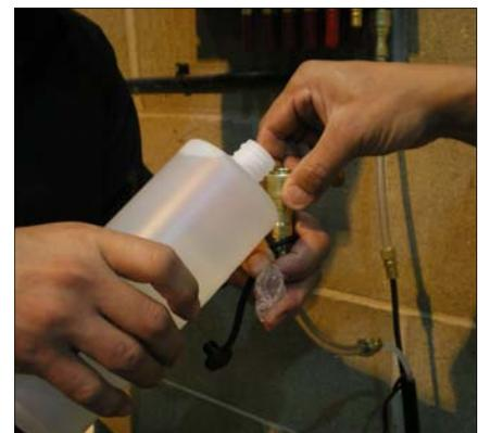
11. Remove the protective cap from the relevant reservoir connector and push on the socket.
